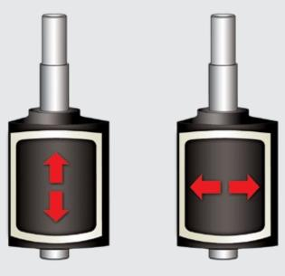
Axial plug movement is not critical to plug/seat alignment or shutoff.
