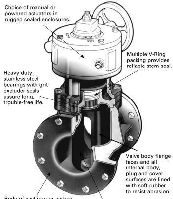
Body of cast iron or carbon steel. Pressure up to 450 psi (3100 kPa). Sizes 3–54" (75–1400mm).
