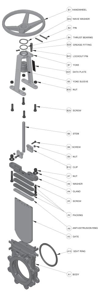
\*The replaceable Seat Ring is standard on resilient-seated valves and optional on metal-seated valves. The standard integral metal seat matches the body material.
