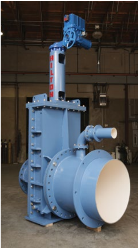
Jet Flow Gate, 24" Inlet, 38" Outlet, 150 psi, CS with 304 SS Trim, Big Tujunga Dam, Los Angeles County
