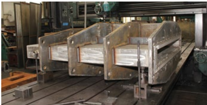
In-House Machining, 72" Bonneted Knife Gate Valve
